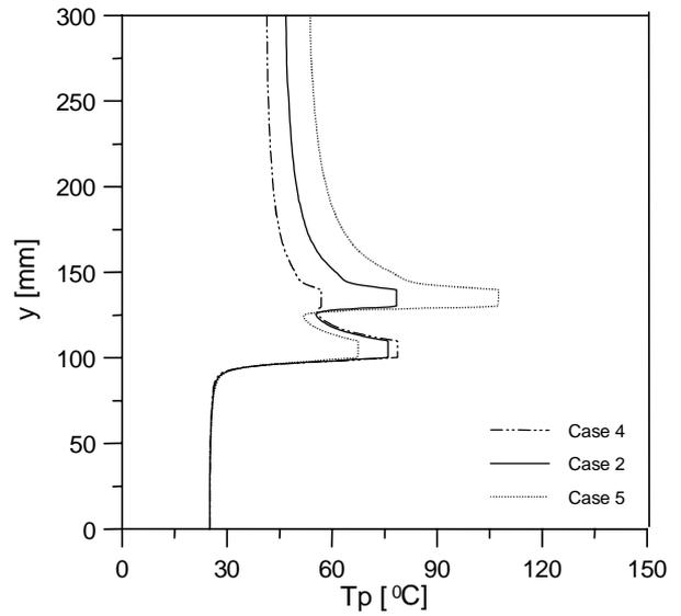
Figure 5: Wall temperature as a function of the power distribution in the sources.
