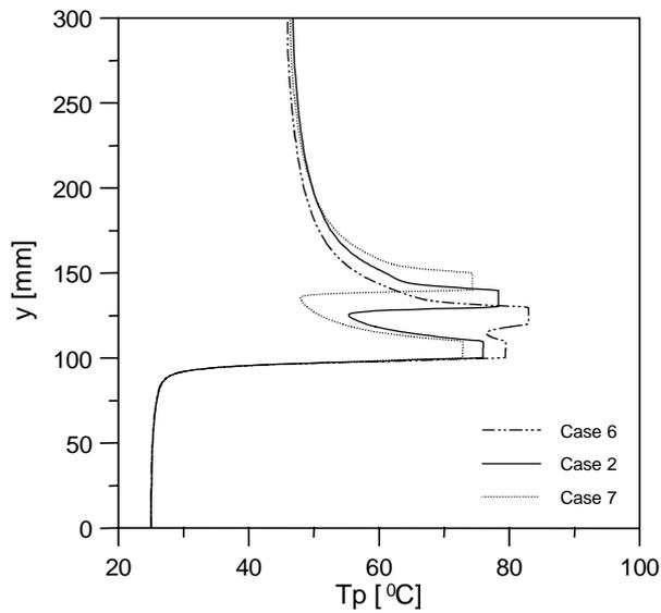
Figure 6: Wall temperature as a function of the spacing between the sources.
