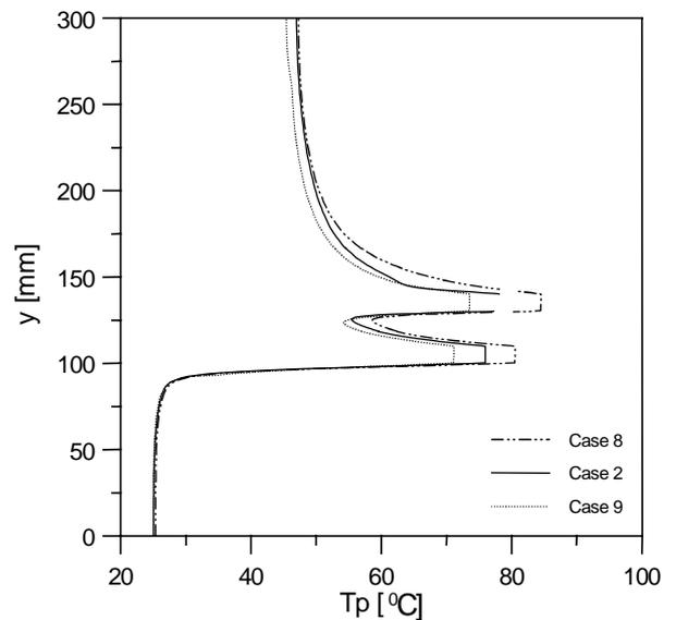
Figure 7: Wall temperature as a function of the aspect ratio of the cavity.
