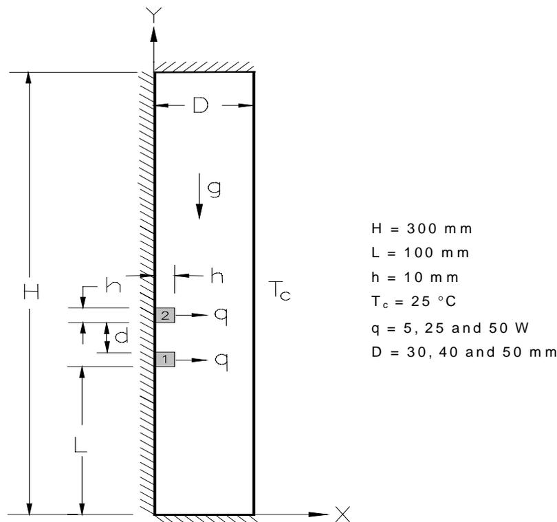
Figure 1: Vertical cavity with heat sources simulating electronic components.
